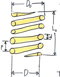
THE WIRE DIAMETER IS & AND THE MEAN TO COLL DIAMETER IS D.
